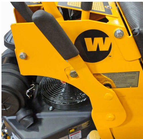
Brake applied, Handlebars locked
